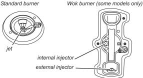
Remove burner caps and heads. Remove old jets. Fit the new jets (see Technical Data section at the back of the book for correct jets). Reassemble in reverse order.
